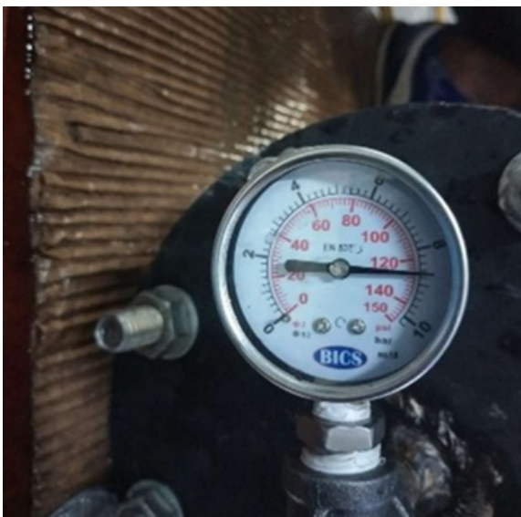
Pressure was increased to over 8 bar after repair and the test rig left for 18 hours. All pipes were inspected with no visible signs of cracks, leaks, deformations or damage - passing the test for use at the complex
