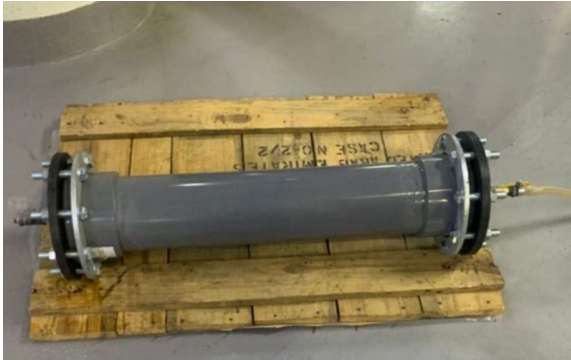
Three ABS pipe test rigs were built with a deliberately weakened flange end. When pressured reached 4 bar, the weak joint began leaking. It could then be repaired using Superfast Aqua PW and SylWrap HD
