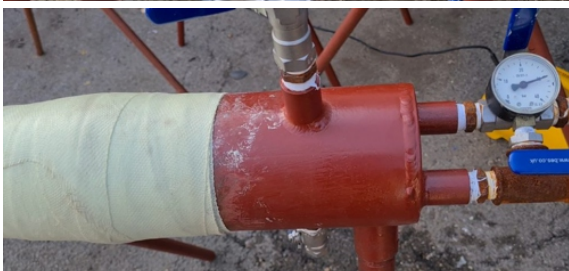
SylWrap HD reinforced the repair, after which it withstood three separate pressure tests up to 30 bar
