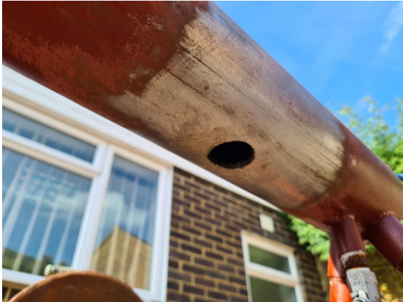
A 25mm hole was cut into the 110mm diameter carbon steel pipe for the qualification test
