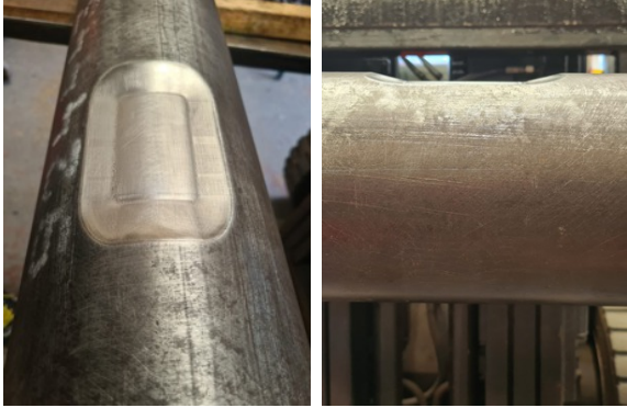
An defect was machined into the pipe spool, reducing wall thickness by 86% to just 1mm
