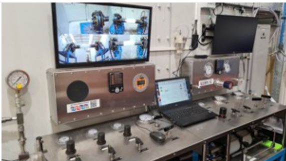
The repair was independently tested and verified to exceed 309.6 bar pressure, qualifying SylWrap HD and Industrial Metal as PCC-2 401-III compliant
