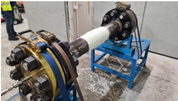
Five SYL633HD Bandages were wrapped over the repair area, creating a hardened shell over 9mm thick
