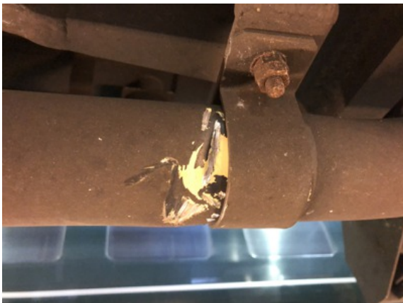
Cables carrying electricity taken from the third rail are housed in aluminium conduit pipe attached beneath the train. The aluminium becomes damaged when stones fly up from loose sections of track bed ballast
