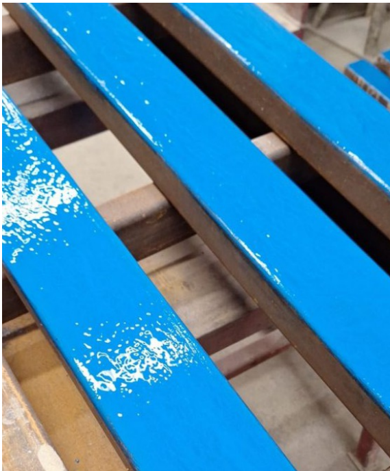
Ceramic Brushable Blue was used to coat the metal slats which came into contact with the abrasive, heavy materials to protect them from future damage
