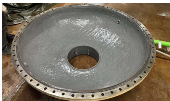
Liquid Metal repaired the heavily corroded metalwork inside the heat exchanger plenum chamber
