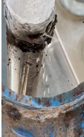
Alcohol juice was spraying through a pinhole leak at a point where the line passed through a circular hole in the upper floor of a platform
