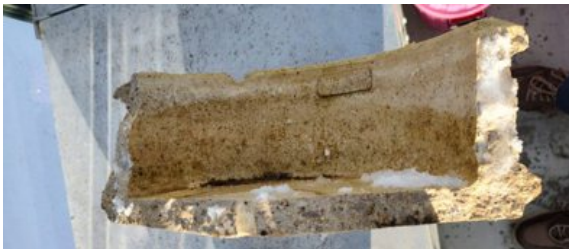
The fountain upper bowl had cracked into pieces due to water freezing inside it through a harsh winter
