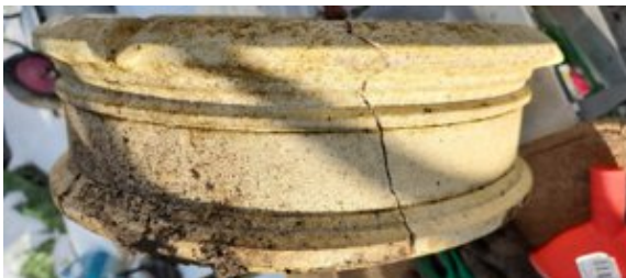
Rapid 5 Minute Epoxy Adhesive bonded the upper bowl back together with remaining cracks and lost sections repaired using AB Original Epoxy Putty
