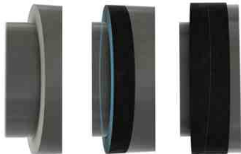
Wrap & Seal application began next to the saddle, was built up until level with the step and then continued across onto the joint
