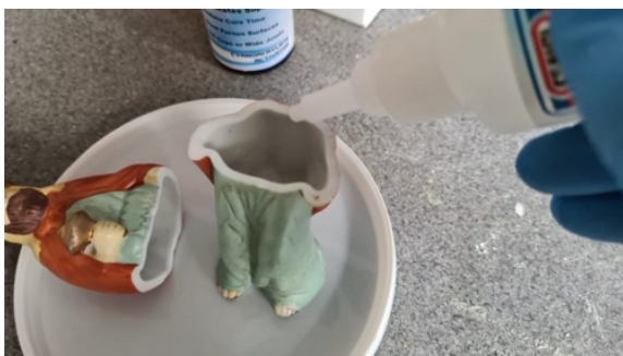
CAE1500 was applied to the lower half of the wise man and the two parts pushed together for around 20 seconds, allowing bonding to take place
