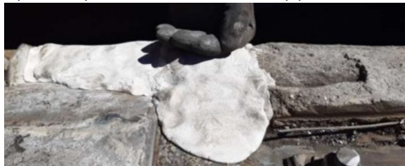
Effluent was escaping from both ends of a failed pipe repair clamp, seen in the centre of the pipe.
