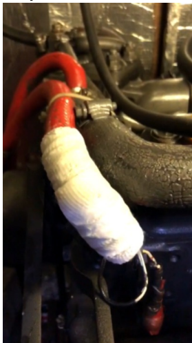
Superfast Steel was applied to the pinhole, followed by a SylWrap HD Bandage to seal the leak
