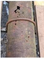
Corrosion had breached the pipe in several places
