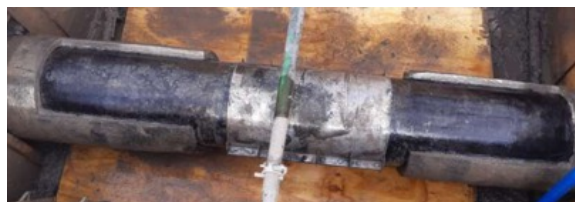
Effluent was escaping from both ends of a failed pipe repair clamp, seen in the centre of the pipe.
