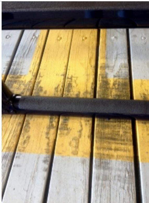
Liquid Metal was coated onto the legs and silicon carbide deposited over the top. Once the epoxy had cured, the grit was permanently bonded to the skids to create a long term anti slip solution
