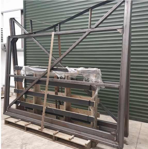
A strong steel frame was built for the replacement gates, onto which wooden slats would be fitted
