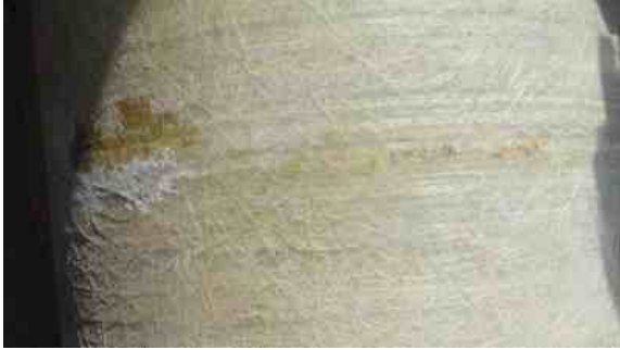
The external surface of the GRP pipe was suffering from heavy scoring which had the potential to lead to future breaches of the line
