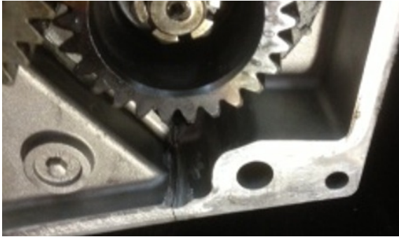
The hairline crack can just about be seen in the centre of the metal casing
