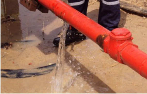
Significant levels of water were escaping the above-ground section of pipe at 5 bar pressure from a longitudinal split
