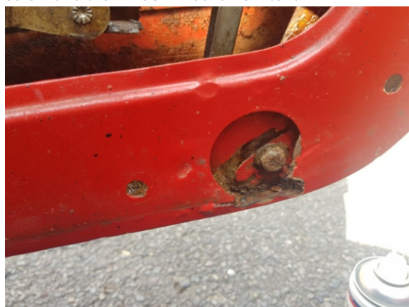
Moisture Repellant Spray was used to drive moisture and grease from the hole. The metalwork was then further cleaned by removing dirt, grime and rust
