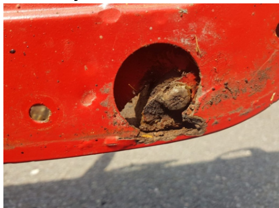
Corrosion had eaten away at the metal frame of the car. It had caused rust holes to develop around a screw and the window mechanism to fail
