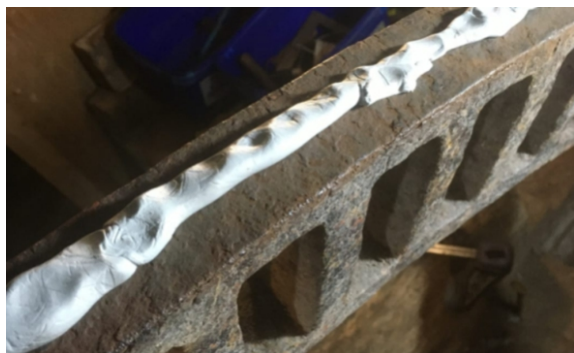
Sylmasta AB applied to the outer casting of the wheel
