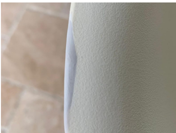
Sylmasta AB bonded to the SMC, filling the chip
